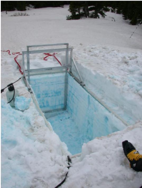
Figure 4. The guillotine instrument after completion of Experiment A (5/23/2003). Dye accumulation along stratigraphic layers is clearly visible in the imaged wall and the sidewall, along with vertical flowpaths between the stratigraphic layers. Note ski boot for scale
