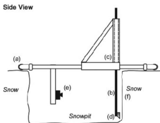
Figure 2. The snow guillotine consists of (a) a stationary PVC frame that rests on the snow surface, (b) a rectangular aluminium cutting frame that moves vertically and (c) a triangular frame that holds the cutting frame perpendicular to the stationary frame. A stainless-steel cutting blade (d) is attached to the bottom of the cutting frame. A digital camera (e) suspended below the PVC frame is used to obtain images of the shaved wall (f) of the snowpit
