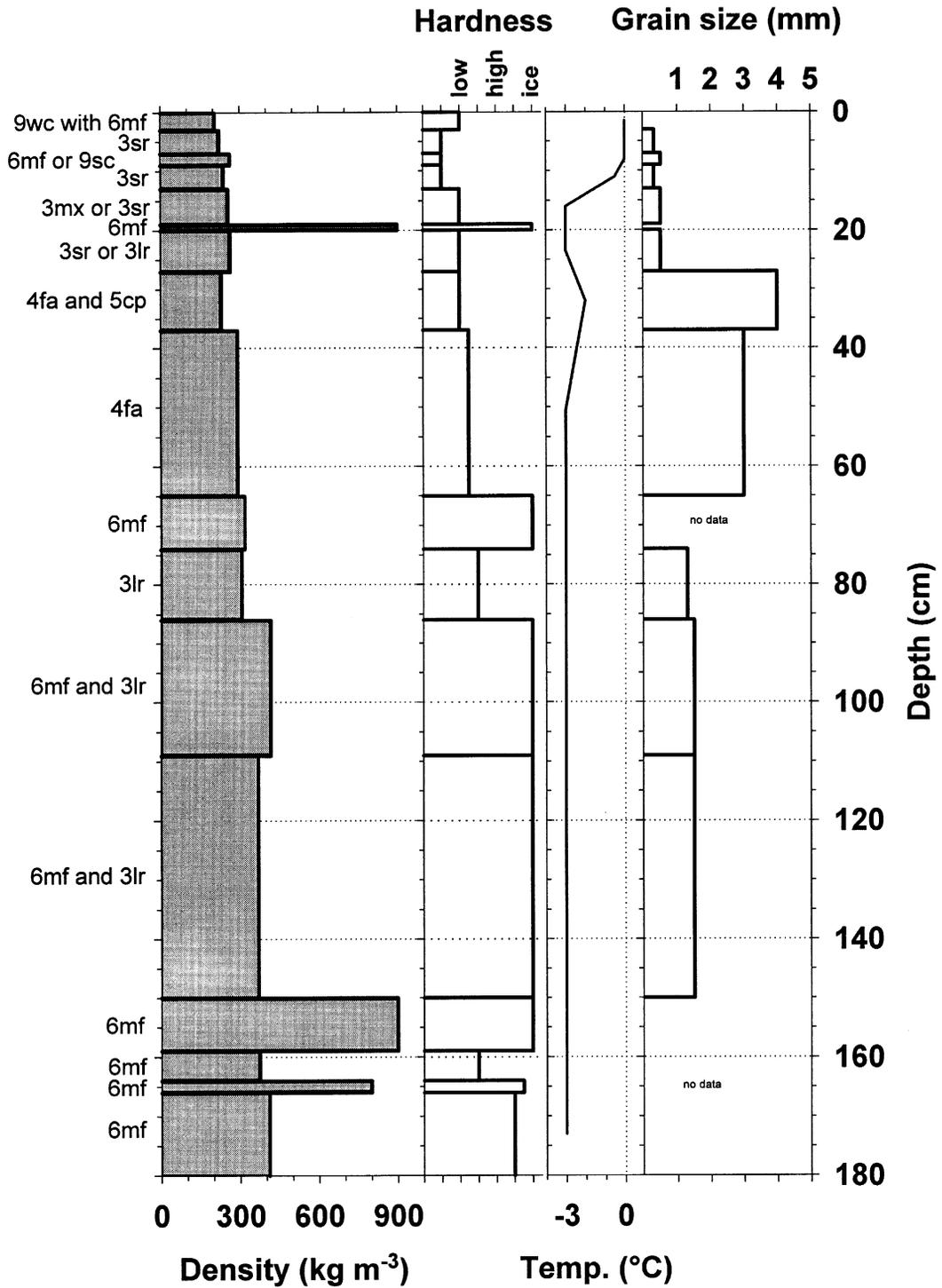
Fig. 4. Snowpit profile sampled at 6300 m near the summit of Nevado Illimani, Bolivia on 30 September 1999. Note the presence of near-surface faceted crystals from 27–64 cm.
