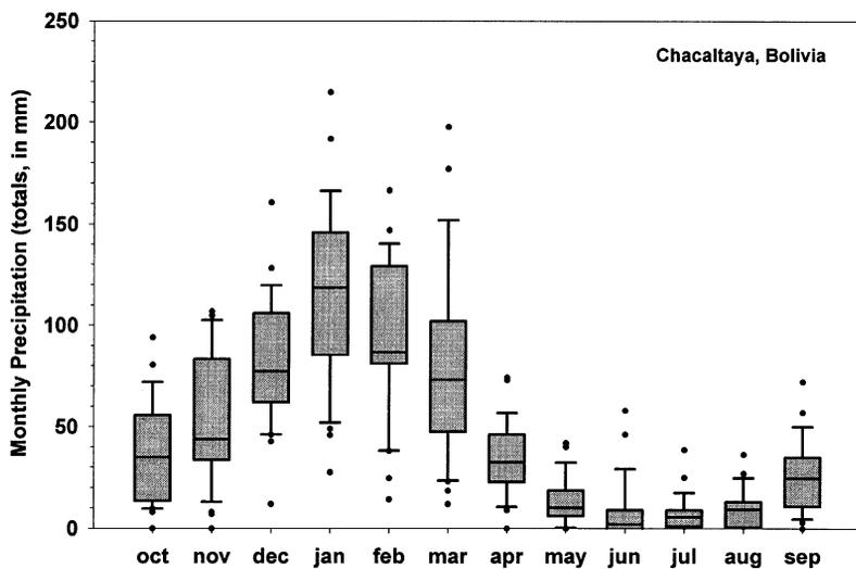
Fig. 3. Monthly precipitation at Chacaltaya, Bolivia (5220 m), 1967–1997. Whisker plot boxes illustrate the median (line) and enclose the 25th and 75th percentiles. Error bars enclose the 10th and 90th percentiles, with extremes indicated by circles. Annual precipitation averaged 560 mm during this period.
