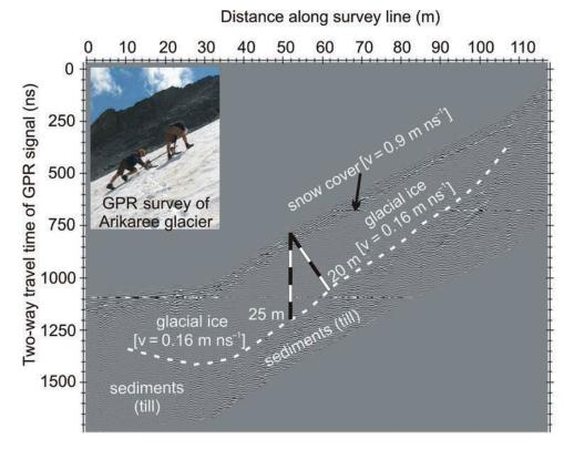
Figure 5. Bottom: Radargram along the indicated line in Figure 4. Glacial ice is represented by a low reflection zone, above the strong reflections from till and probably bedrock. On top the recent snow cover, partly compressed, is indicated by strong reflections parallel to the slope. Glacial ice thickness reaches 25 m as a maximum. The inset image shows GPR data collection during the summer of 2009.
