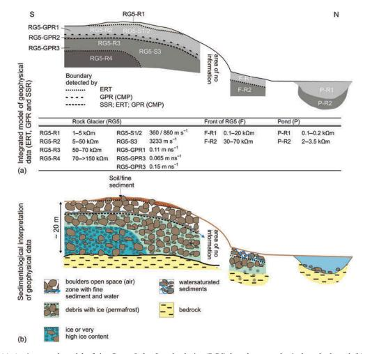
Figure 10. (a) An integrated model of the Green Lake 5 rock glacier (RG5) based on geophysical methods and (b) an interpreted stratigraphic model of the internal structure of the rock glacier. GPR, Ground-penetrating radar; ERT, electrical resistivity tomography; SSR, shallow seismic refraction; CMP, common midpoint (from Leopold et al. 2011, modified). *Reproduction under License Number* 3547521009552, 14-Jan-2015, John Wiley and Sons
