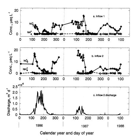
*Fig. 5.* Concentrations of  $NH_4^+$  and  $NO_3^-$  from inflow 1 (panel a), inflow 2 (panel b) and discharge from inflow 2 (panel c), 1986–1988.
