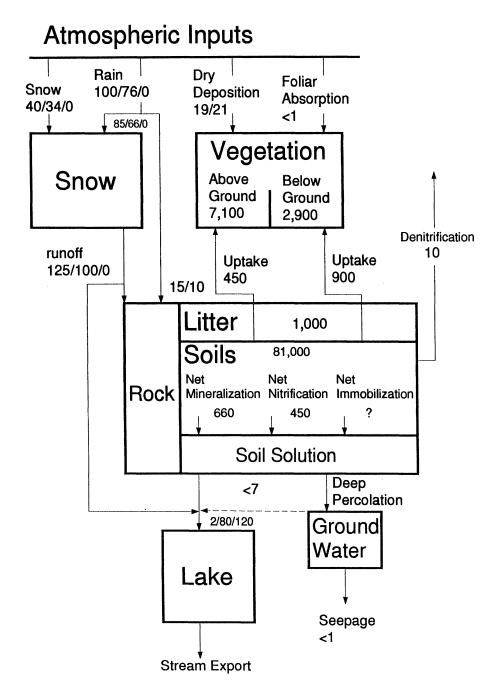
*Fig. 6.* Conceptual mass balance of nitrogen pools and fluxes, water year 1987. Pools are eq ha<sup>-1</sup> and fluxes are eq ha<sup>-1</sup> yr<sup>-1</sup>. Single values are total N; where possible N values are separated into  $NH_4^+/NO_3^-/TN$  minus inorganic N.
