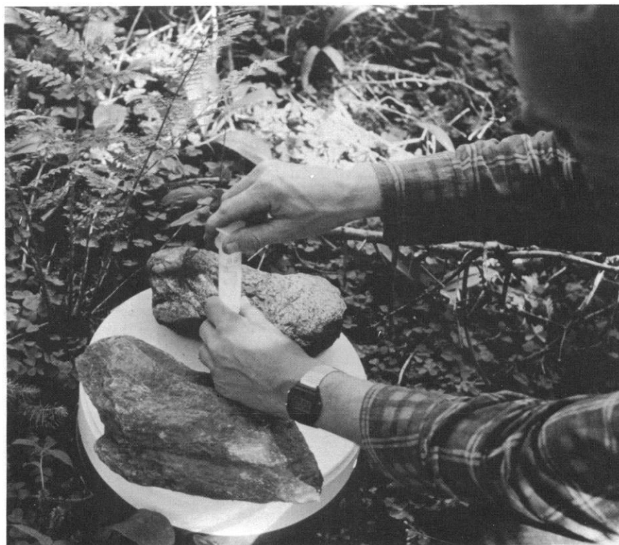
Figure 6. Soil chambers used for measurement of methane and nitrous oxide fluxes from forest soils. Chamber sits on rim pressed firmly onto soil surface, but not penetrating the soil or severing roots. Access port on cover allows extraction of headspace gas samples.
